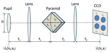
Figure 1. Schematic representation of the P-WFS.
