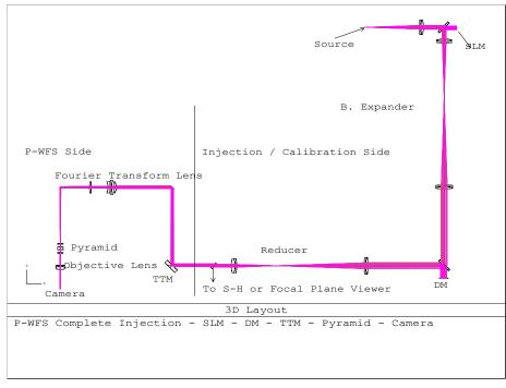
Figure 5. Optical layout of the pyramid wavefront sensor test-bench.
