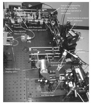
Figure 2. First iteration P-WFS test-bench (single wavelength).
