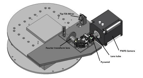
Figure 9. Bottom view of the Mont-Mégantic adaptive optics test box with all P-WFS components.
