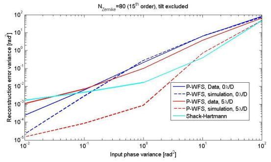
Figure 4. Reconstruction error variance of the P-WFS as a function of input phase variance based on 80 Zernike coefficients.30 images (at 60 fps) co-added for each point. Comparison with the simulated Shack-Hartmann performance.
