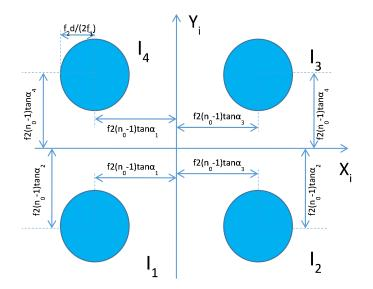
Figure 7. P-WFS system generates four images of the pupil plane; position of each image is function of the pyramid angles.
